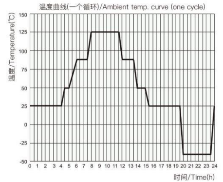
电耐久性试验环境温度曲线 Ambient temperature curve of the electrical endurance test
